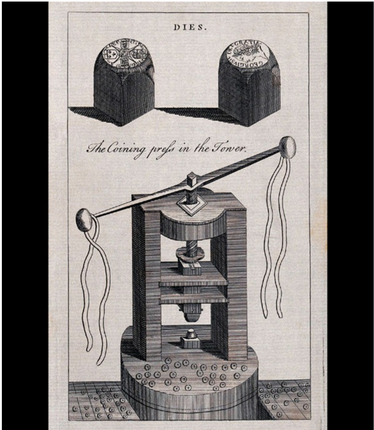
A diagram of a coining press and dies found in the Tower of London, 1800. Until 1812, the Tower of London was the site of the Royal Mint, where most British coins were made.
